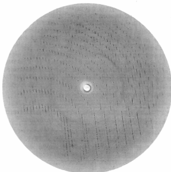
Fig. 3. A screenless rotation photograph from a crystal of the heterologous complex of E. coli AspRS and yeast tRNA Asp obtained in ammonium sulfate, recorded at 113 K on an MAR Research imaging plate using the X11 beamline of DESY. The oscillation range was 0.5° and the exposure time 360 s. The crystal-to-film distance was 400 mm, giving a resolution limit of 2.6 Å at the edge of the photograph.
